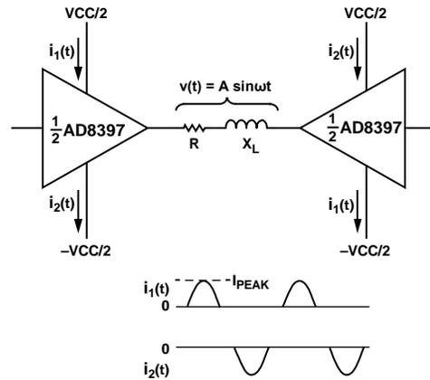
Figure 14. Equivalent Circuit for Calculating Power Supply Current
