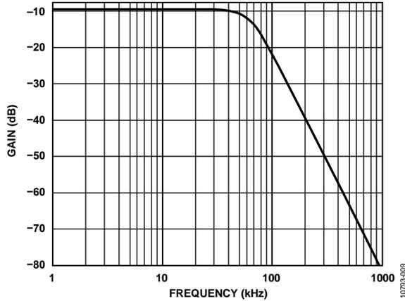
Figure 9. Resolver Receiver Circuit, Low Gain Transfer Function
