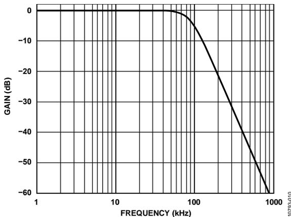
Figure 10. Resolver Receiver Circuit, High Gain Transfer Function
