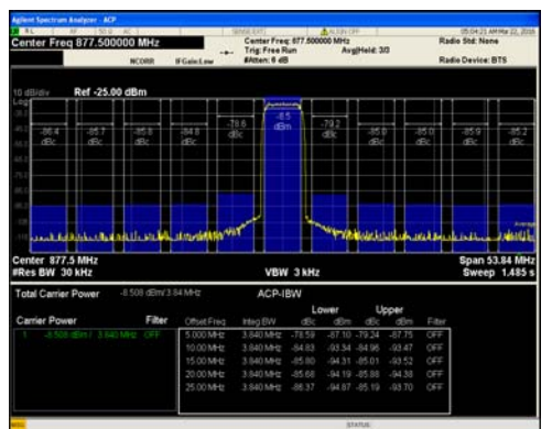
Figure 84. Single-Carrier W-CDMA at 877.5 MHz
