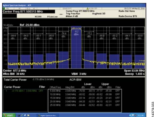
Figure 25. Single-Carrier W-CDMA at 877.5 MHz
