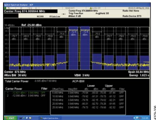
Figure 27. Two-Carrier W-CDMA at 875 MHz
