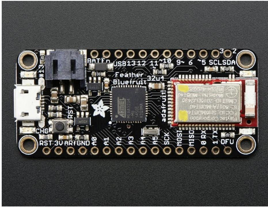
At the Feather 32u4's heart is an ATmega32u4 clocked at 8 MHz and at 3.3V logic, a chip setup we've had tons of experience with as [it's the same as the Flora](https://adafruit.it/dVI) (<https://adafruit.it/dVI>). This chip has 32K of flash and 2K of RAM, with built in USB so not only does it have a USB-to-Serial program & debug capability built in with no need for an FTDI-like chip, it can also act like a mouse, keyboard, USB MIDI device, etc.
